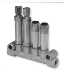
Positive Displacement Units (PDU's) deliver a precise volume of lubricant at the beginning of each pump cycle. Each unit in the range is stamped with a reference number denoting the discharge volume. The total oil delivery to a system can be further controlled by the pump lubrication frequency. The system operates intermittently, allowing PDU's to recharge for the next cycle, and is generally total loss.
